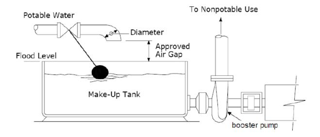
Note: Air gaps must be twice the diameter of the inlet pipe, at least 1", but no greater than 12."
