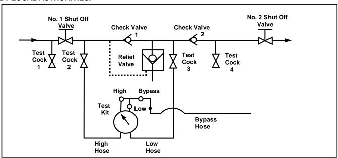
**TEST SET UP:**
